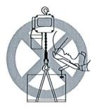
Forbidden to do welding or cutting operation when the weight was lifted in the air.
