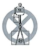
Lifting weight can not over the rated lifting capacity.
