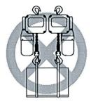
Forbidden to use multi pieces of hoists to lift weight which is over the rated capacity of the single hoist.
