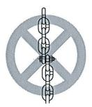
Do not use bolt, screw driver etc to knot or shorten the lifting chain
