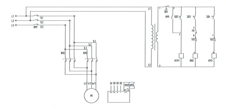
$\mathbf{2}$  single lifting speed single traveling speed type electric schematic diagram
