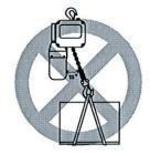
Do not lift the goods slant the angle can not over 12 than vertical direction
